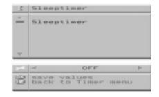
→ Use the **Volume** keys to select the desired time period (1...240 minutes) in steps of one minute at a time, then press the **OK** key to store in memory.
